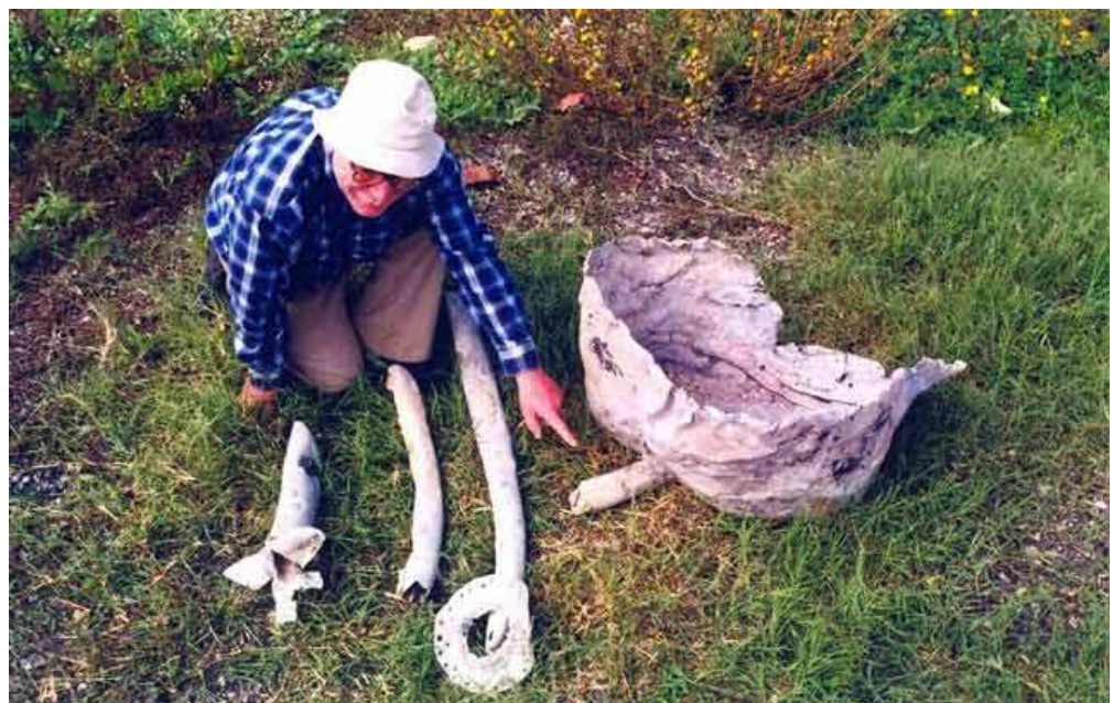
2. Lead pipes and a lead collecting box of a bilge pump.
