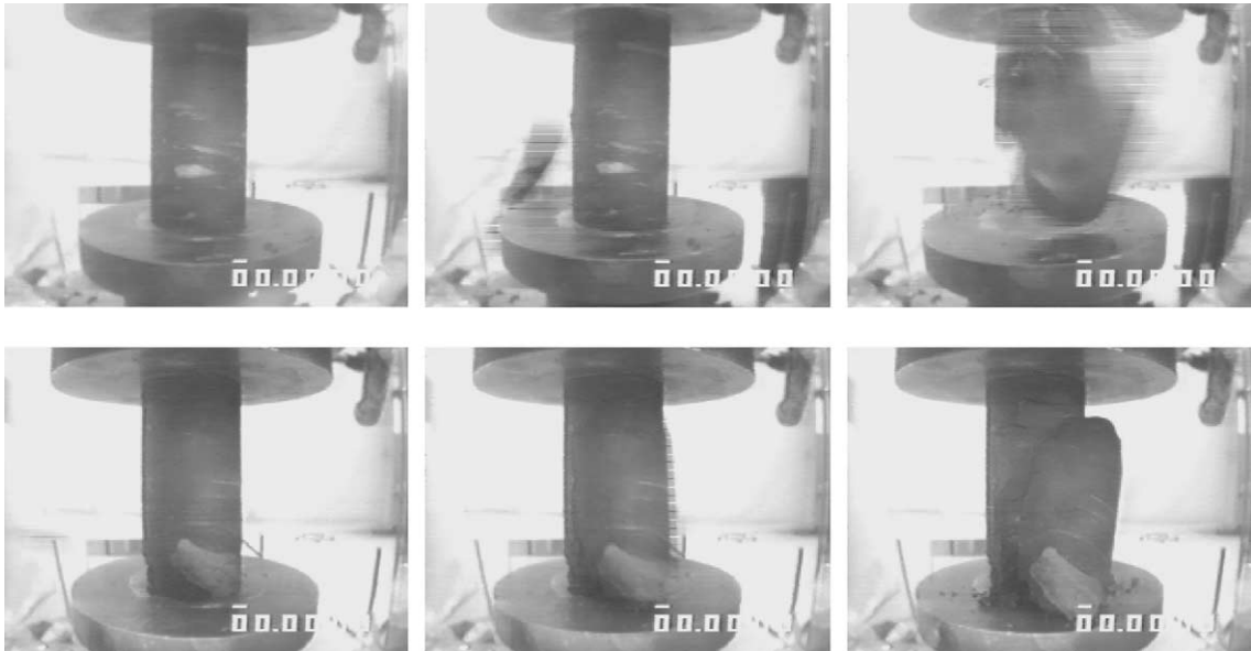
Fig. 24. Main stages of fracture of (a) real lignite specimens under uniaxial compression, (b) specimens fracture.
