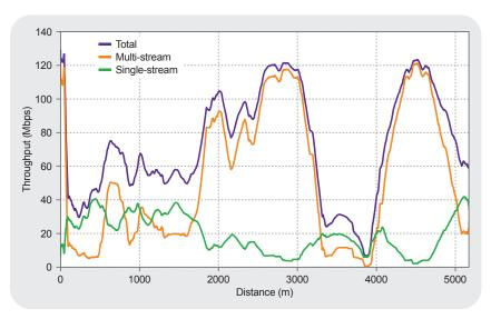
Figure 11. DL throughput on long distance route for single-stream and multi-stream transmission
