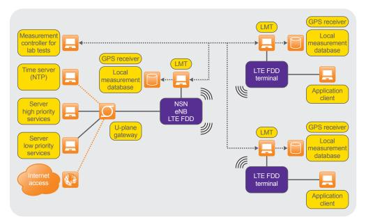
Figure 1. Nokia Siemens Networks LTE development platform
