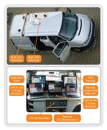
Figure 2. Measurement van with LTE UEs
