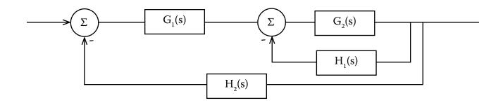
To obtain the forward path of the major loop, we just overlay plots of  $G_1(s)G_2(s)$  and  $G_1(s)$ .  $\frac{1}{H_1(s)}$ . The forward path is the lower of the two curves at all frequencies
