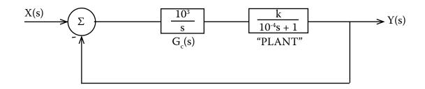
The problem is that k can range anywhere from  $10^1$  to  $10^2$ ! Calculate the phase margin and loop crossover frequency at the two extremes.
