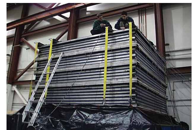
Fig. 35: Laminar Soil Box on a Shake Table
