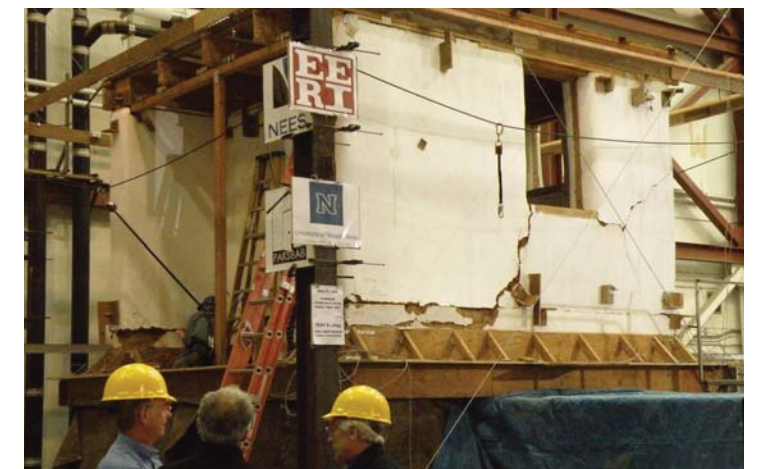
Fig. 18: The Straw Bale House Survived Two Times the Northridge Earthquake
