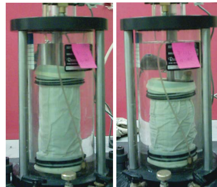
Fig. 22: Soil in a Liquefied Condition in Extension (left) and Compression (right)
