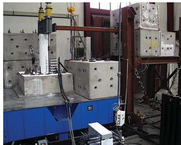
Fig. 5: The Off-Table Mass Rig Attached to a Column on the Shake Table
