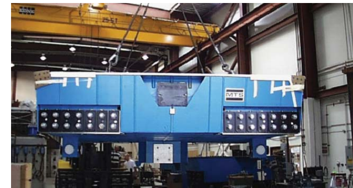
Fig. 6: Installation of the Third Biaxial Shake Table, 2001
