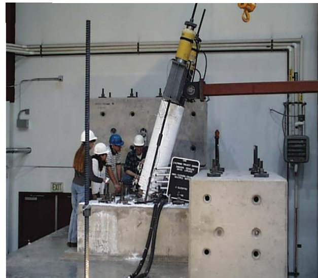
Fig. 4: A Column under Test on a Shake Table in the Large-Scale Structures Laboratory
