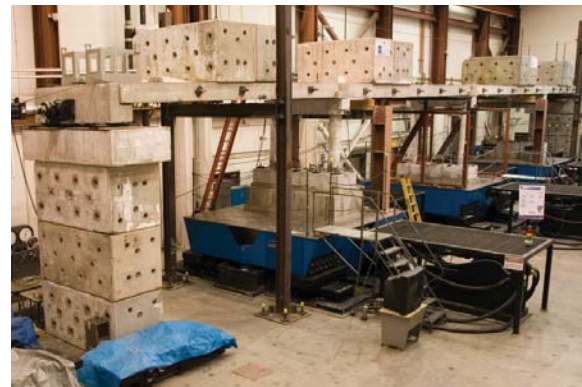
Fig. 7: Four-Span Bridge on Three Shake Tables and Two Abutments with Servo-Controlled Actuators
