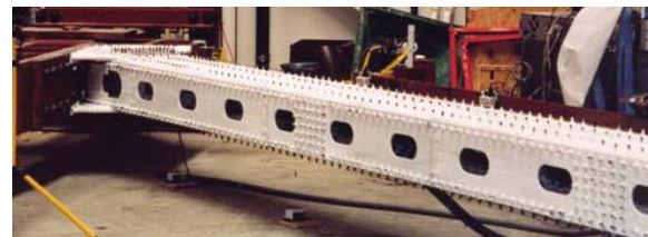
Fig. 15: Perforated Members in the SFOBB
