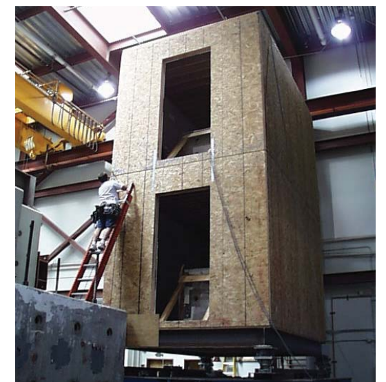
Fig. 19: Full-Scale Isolated Two Story Timber Building on a Shake Table
