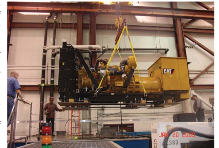
Fig. 25: Lifting an Electric Power Generator onto a Shake Table
