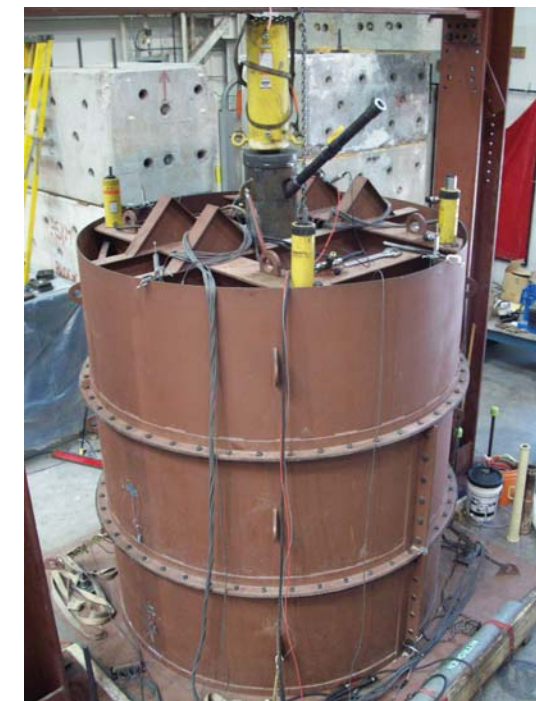
Fig. 21: Post Grouted Pile Test Setup
