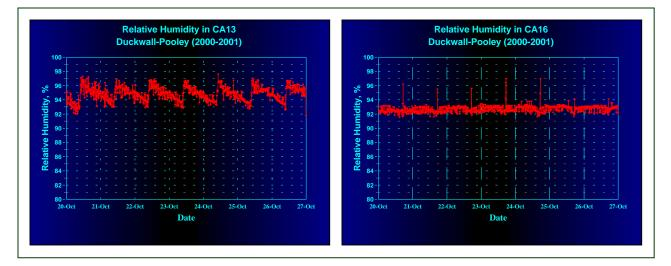
Mode 3 operation induced a 1.5 °F drop in ammonia temperature during the fan on periods, which included intentionally lowering the room set point 0.3 °F. During the fan cycling period, room relative humidity ranged from 96% to 92% in CA 13 and from 92% to 89% in CA 16. The high values were recorded during fan off periods.
