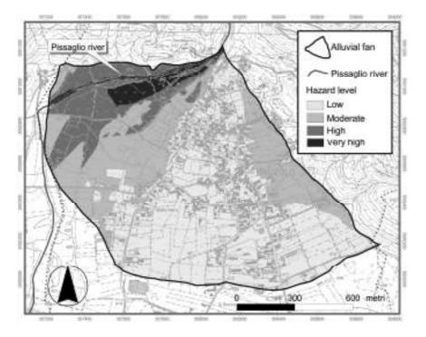
Figure 5. Bruzolo alluvial-fan hazard zonation. The Pissaglio river follows the path resulting from river engineering structures.
