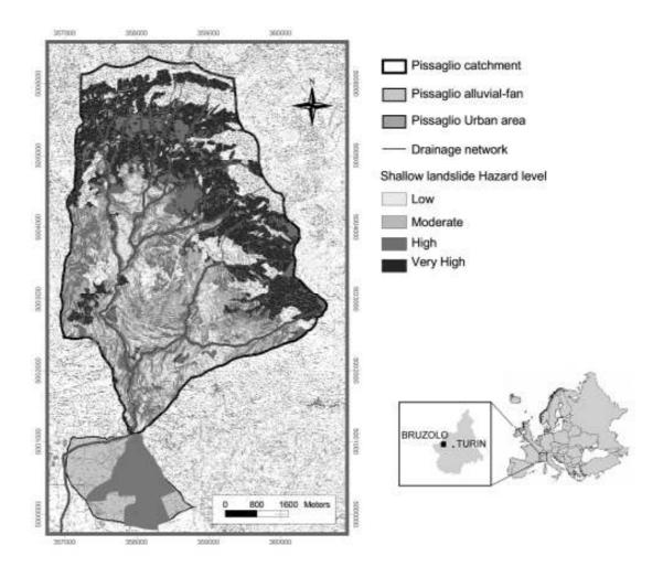
Figure 4 – Shallow landslide hazard assessment – Results. Potential sediments sources are represented by very dark and dark areas, where shallow-landslide hazard is high or very high. The analysis does not include outcrops.
