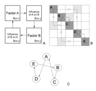
Figure 1. Example of a Binary interaction matrix (BIM) and hypothetical pathway for a 5-factor BIM; after Jiao and Hudson (1995).
