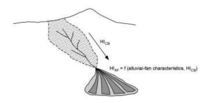
Figure 2. Alluvial-Fan Hazard evaluation: hazard level is calculated considering both alluvial-fan features and upstream catchment proneness to deliver sediment to downstream areas.
