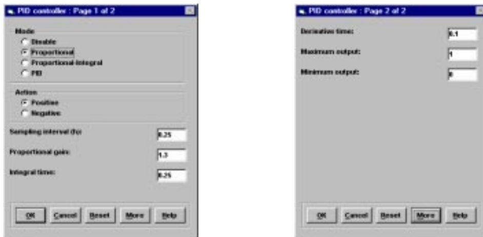
Figure 10.6: Nitrate PI controller settings.
