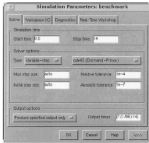
Figure 8.2: Explicit results output times have been specified in the simulation parameter window. Results are saved from day 7 to day 14 with a time interval of 1/96 day = 15 minutes.
