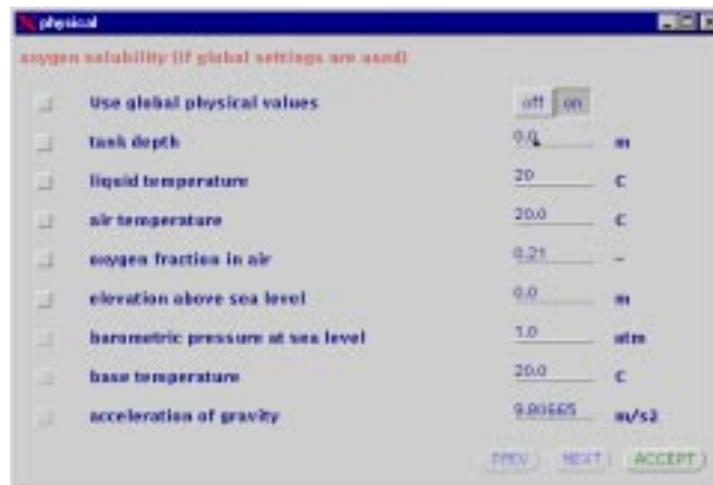
Figure 7.5: The GENERAL DATA menu 'physical' dialogue box showing the required DO parameter values to achieve a DO saturation concentration of 8 \text{ g m}^{-3} .
