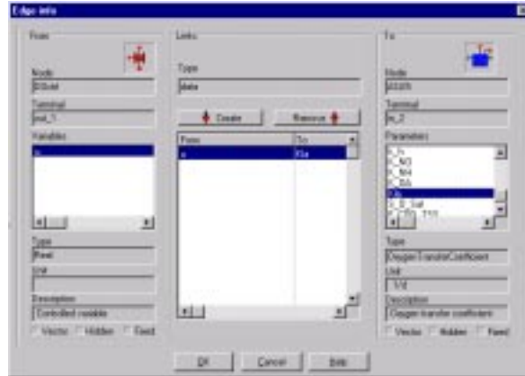
Figure 11.7: Connection specification window showing the linkage of the DOctrl PI-controller's output to ASU5 's K_La parameter.
