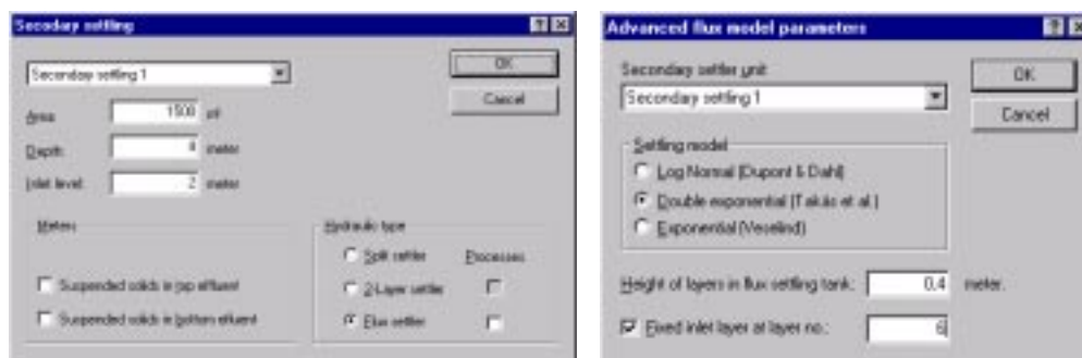
Figure 5.3: 'Secondary settling' and 'Advanced flux model parameters' dialogue boxes used to input the settler characteristics.
