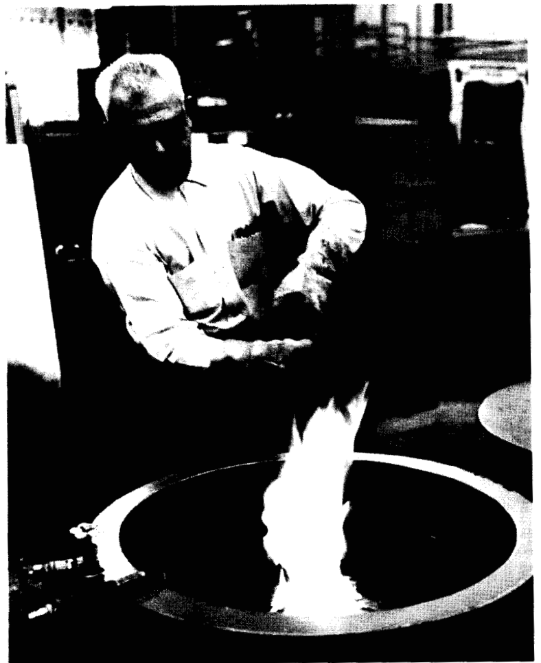
Wiley Jenkins, metal fabricator supervisor in the Sheetmetal Branch, is heat-treating steel in the oil quench tank, a procedure reminiscent of the blacksmithing art.
