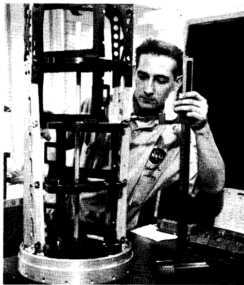
Bob Hessler, of the Machine Branch, is checking the alignment of the stellar spectrometer bases in a rocket's payload frame.
