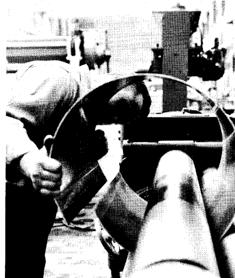
Burton Kelbaugh, aviation metalsmith, forms a 20-inch diameter aluminum cylinder on the metal rolling machine.
