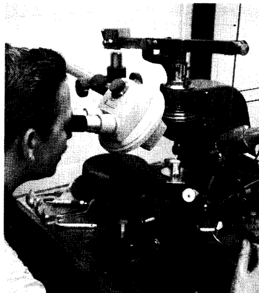
William R. Gotthardt, machinist, drills a hole measuring one-quarter the breadth of a human hair in part of an ultra-precision spectograph.
