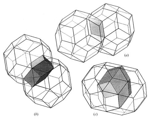
Figure 3. Two rhombic triacontahedra sharing (a) a single oblate unit, (b) a rhombic dodecahedron, and (c) a rhombic icosahedron.
