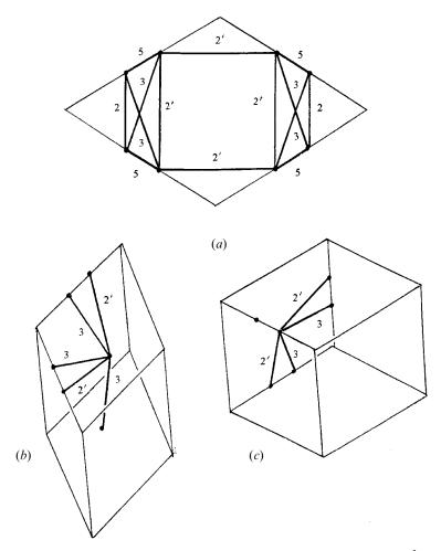
Figure 4. Lines of centres for overlapping pairs of 30-hedra, occurring in the  $\tau^3$  units: (a) a face of a  $\tau^3$  unit (edge length is  $\gamma\tau^3$ ); (b)  $\tau^3$  prolate unit; and (c)  $\tau^3$  oblate unit. Bonds that have been omitted for clarity are obtained from those shown by the  $\bar{\mathbf{3}}$  symmetry of the unit.
