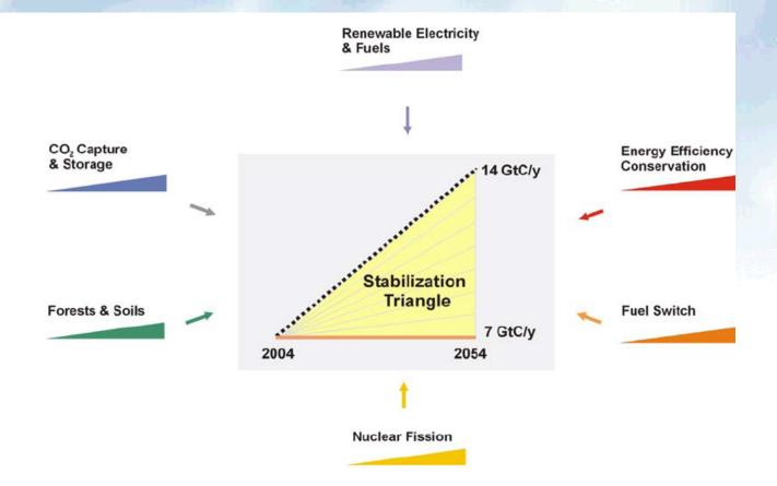
gure 2: Filling the Stabilization Triangle with seven "wedges." Six broad categories are identified.
