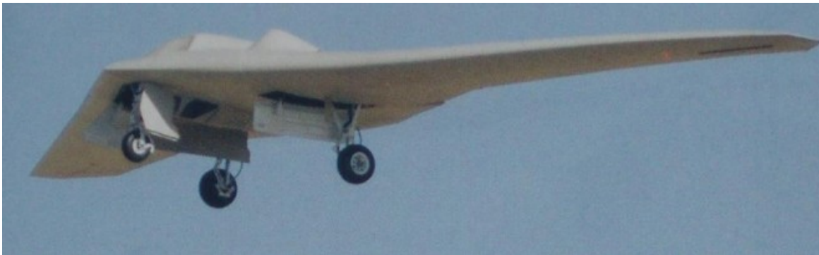
Figure 41. Lockheed-Martin RQ-170 Sentinel Stealth Unmanned Aerial Vehicle (UAV) drone, known as the Beast of Kandahar. Source: Lockheed-Martin.
