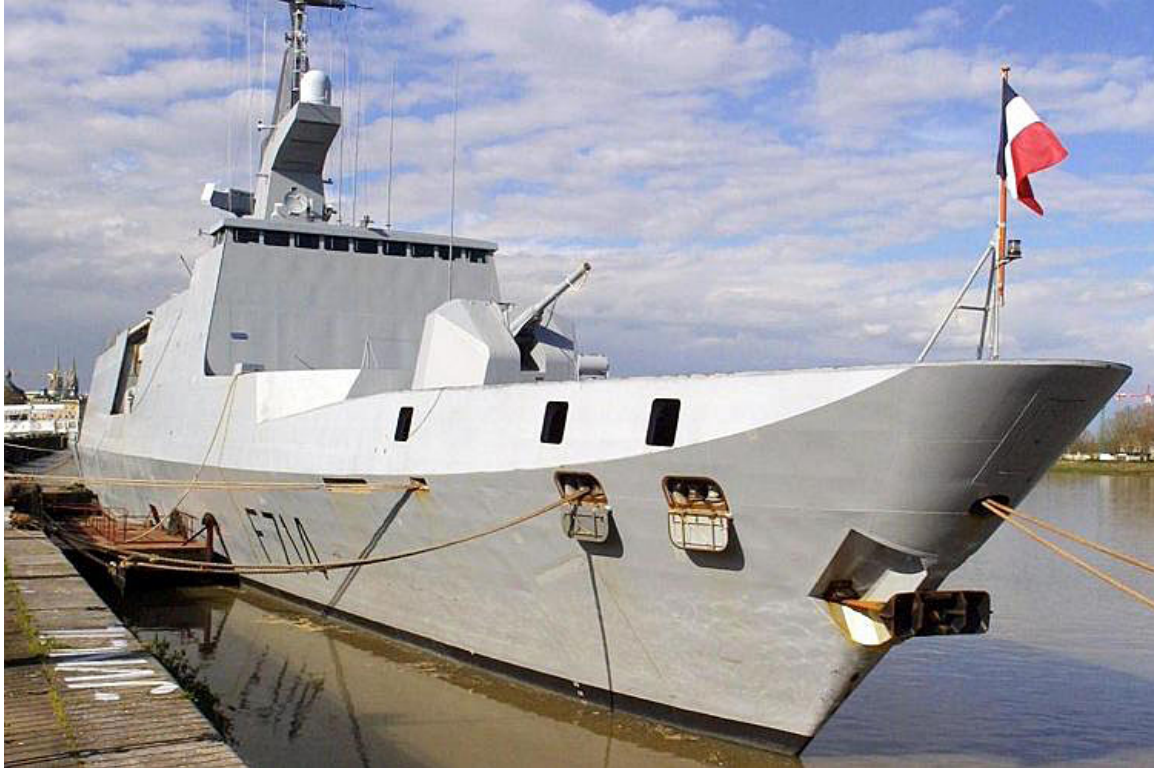
Figure 43. Stealth radar deflecting technology implemented into a French Lafayette class frigate, 2001.
