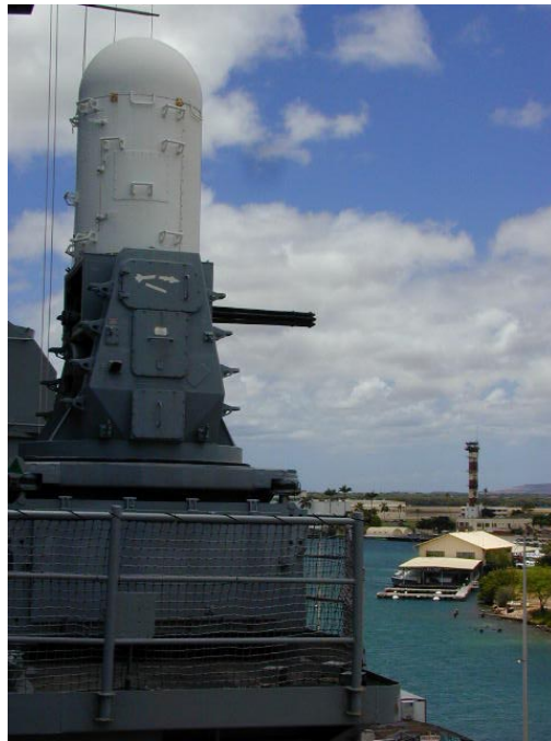
Figure 18. The Phalanx radar-guided gun, nicknamed as R2-D2 from the Star-Wars movies, is used for close-in ship defense. The radar controlled Gatling gun turret shooting tungsten armor-piercing, explosive, or possibly depleted uranium munitions on the USS Missouri, Pearl Harbor, Hawaii. Photo: M. Ragheb.
