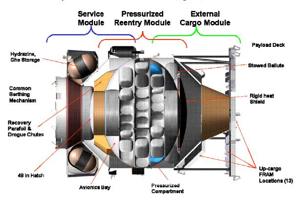
Figure 3. ARCTUS is composed of three primary elements, the external cargo module, pressurized reentry module, and the service module
