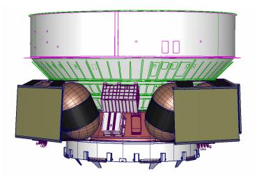
Figure 6. ARCTUS Aft Service Module houses the propulsion and avionics systems.
