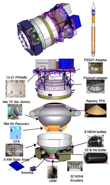
Figure 2. ARCTUS is primarily derived from existing, flight qualified components that are currently in production
