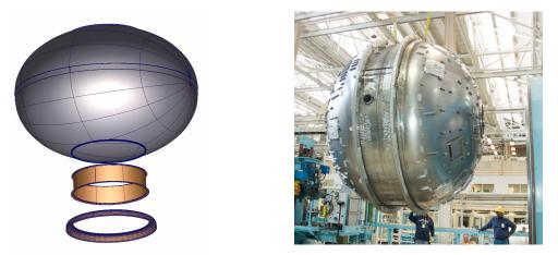
Figure 5. The ARCTUS Pressurized Reentry Module is built from 2 Centaur domes.
