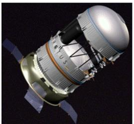
Figure 13. ARCTUS can support propellant resupply of orbiting fuel depots.
