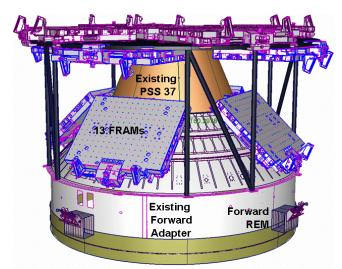
Figure 4. The ARCTUS Forward External Cargo Module enables carriage of large, oversized ORU's such as the rate moment gyros.
