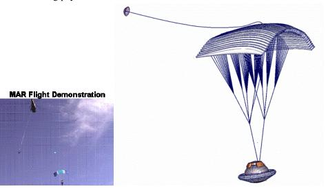
Figure 10. Mid Air Recovery provides very benign environments for the returning cargo.
