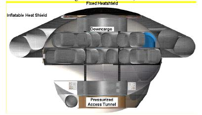
Figure 8. ARCTUS Pressurized Cargo Accommodations provide 400 ft<sup>3</sup> of conditioned payload volume supporting both up and down mass.
