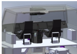
Pilot/Co-Pilot Dual Controls New C4N suite
