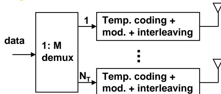
**Horizontal Encoding (HE) :** div. order =  $N_T$ ; sub-optimal; easy to decode
