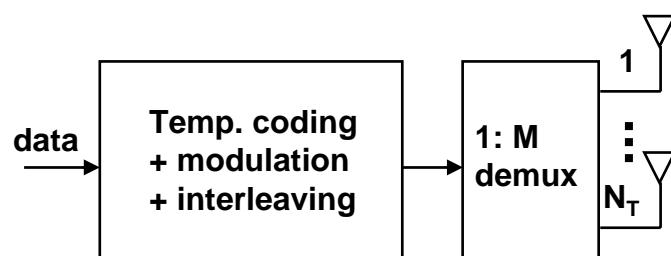
**Vertical Encoding (VE) :** div. order =  $N_T N_R$ ; optimal; require joint decoding of streams
