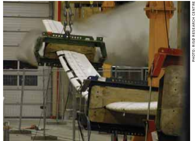
FIGURE 9.1 Full-scale testing of a wind turbine blade at Risø National Laboratory. Risø's test station for wind turbines was established in 1978 with the aim of developing new opportunities for industry and society in the exploitation of wind power.
