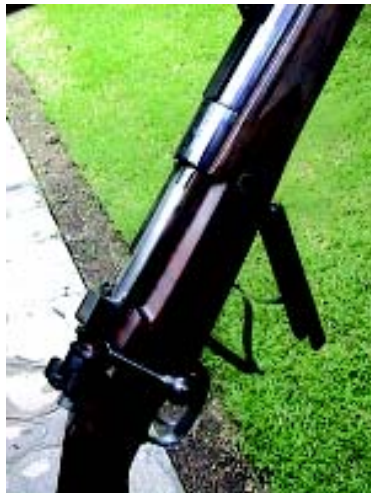
After three shots the magazine floor plate started springing open on every shot.
