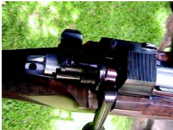
After 10 shots the recoil caused a small piece of the stock to break off.
