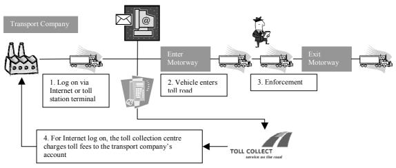
Figure 10: Manual log-on Source: Toll Collect GmbH
