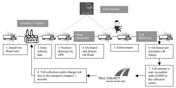
Figure 9: Automatic log-on Source: Toll Collect GmbH
