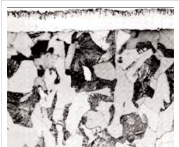
Figure 8A SAE 5115, chrome-manganese low carbon steel, LNC treated 90 minutes, 1075°F Original magnification 500X Nital etch
