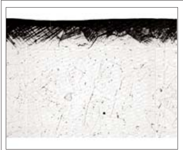
Figure 11A 304 stainless, steel, LNC treated 90 minutes 1075°F Original magnification 500X Complex etchant
