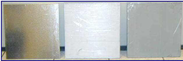
Pictured above are examples of three tile finishes. The spangled surface (left) and the light gray, streaked surface (middle) are both hot-dipped. The uniform dull gray surface (right) of the electroplate tile is also apparent.
