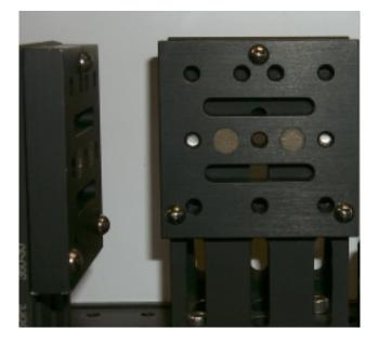
FIGURE 7.10 KINEMATIC MOUNTING UNIT
