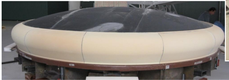
Heat Shield Carrier Structure Fabrication
