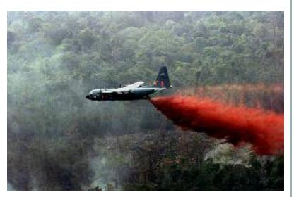
Air National Guard C-130 Hercules equipped with modular airborne firefighting systems, similar to this one, are dropping thousands of gallons of retardant on the wildfires in Southern California. The fires have destroyed more than 830 homes and burned out more than 500,000 acres. California officials said the fires are responsible for at least 15 deaths. (U.S. Air Force photo by Staff Sgt. Daryl McKamey)
