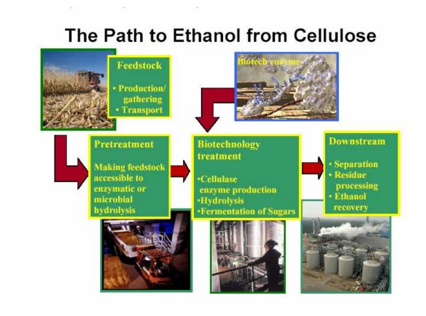
Recent advances in the relatively new field of industrial biotechnology are making it possible to convert cellulosic biomass to ethanol. Enzymes that break down cellulose – called "cellulases" – can economically convert plant matter to fermentable sugars. Cellulases are naturally produced by fungi as well as microbes, such as those from the guts of termites. Biotech tools are necessary to identify or produce the most efficient cellulases on a scale useful for ethanol production.
