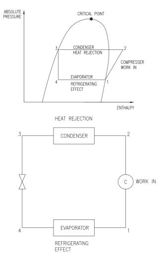
Fig 5. Coefficient of Performance
