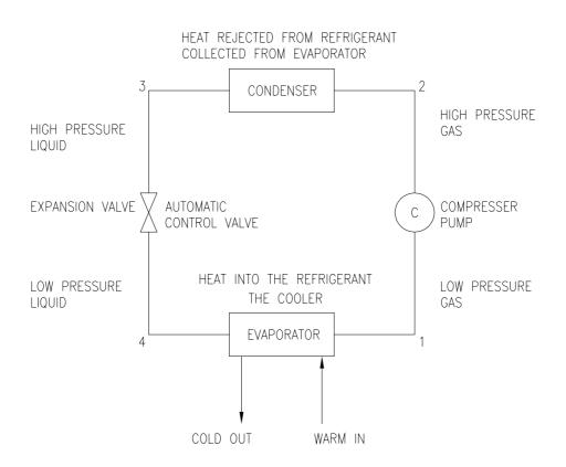
Fig 6. The Refrigeration System
