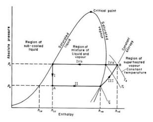
Fig. 2. Refrigeration P-H Diagram
