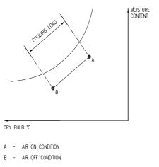
Fig 3. Cooling Load
