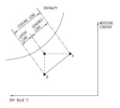
Fig 4. Sensible and Latent Cooling Loads
