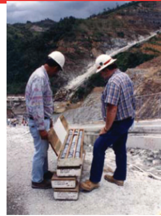
Corps geologists examine rock samples from borings to analyze the effectiveness of the drilling and grouting program.
