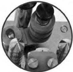
The head-stack for Magnetic Film Transports features special guide-rollers and pins. Pinch rollers ensure a tight film to head contact. It becomes possible to playback even worst deformed and shrunk magnetic tracks.
