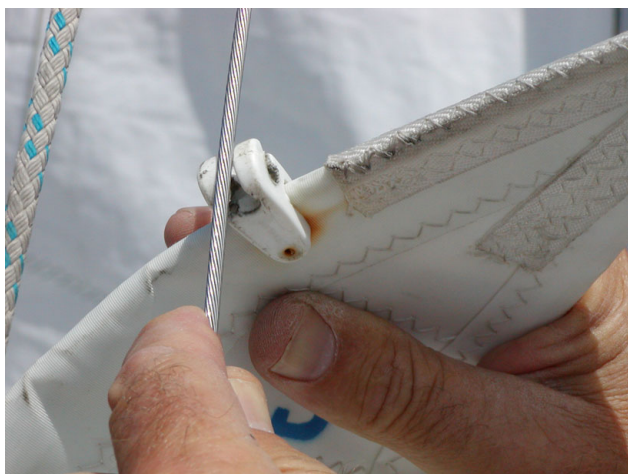
19. Attach the hanks on the jib luff to the forestay.
