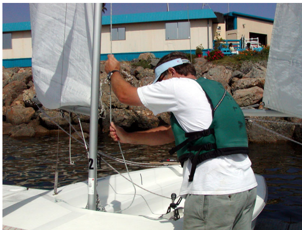
21. Lead the jib sheets through the fairleads OUTSIDE the shrouds, and secure them by tying a figure eight stopper knot close to the end of each sheet (refer to page 28). NB: At least six inches of line should be free at the bitter end (extreme end of a line).
