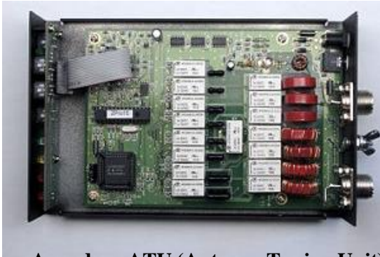
A modern ATU (Antenna Tuning Unit) for ham operators
