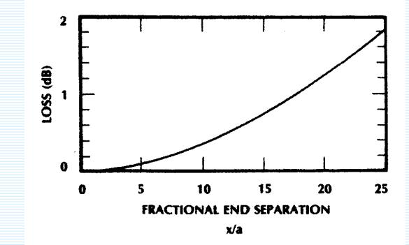
End- separation loss for single mode SI fiber V=2.4, w/a=1.1,NA=0.12and  $\lambda = 0.8 \mu m$
