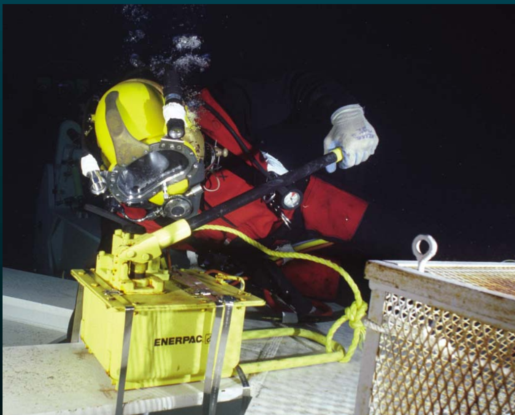
Surface supplied diver operating hydraulics on turret lifting system spider. Photo by Fleet Combat Camera, Atlantic.
