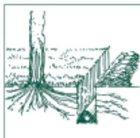
Trenching Near Trees Avoid trenching near trees whenever possible. If unavoidable, make clean cuts on roots and keep moist until backfill is complete.
