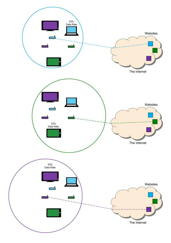
And, the problem only grows worse with more users. In a city building, it is common to see 25 Wi-Fi networks or more listed on a user device. If all of the networks are sharing the same spectrum optimally, each user will only get 1/25<sup>th</sup> (4%) of the data rate. As users are added, the data rate per user steadily decreases.
