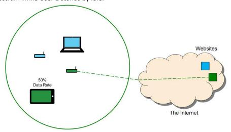
If we assume the protocol divides up the spectrum evenly between the two APs, then each user optimally will get 50% of the available bandwidth. So, when two Wi-Fi users are in range, each user loses half of the data rate they would have had alone. As we add more users and APs at the same frequency within range of Users 1 and 2 and APs 1 and 2, then we see a steady decline in available data rate per user.
