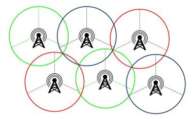
But as mobile usage grew exponentially, both in number of users and the amount of data, it began to tax the cellular system. Improvements were made, such as dividing cells like a pie into sectors, and utilizing more advanced digital transmission techniques such as MIMO. But, despite these advances, a given cell
