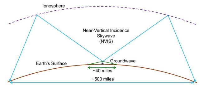
A key limitation for data communications using the HF bands that work with NVIS is that they are very narrow and a large percentage of the HF band would have to be used to provide sufficient data rate for broadband applications to even one user in the entire 500-mile area. Of course, DIDO would be an ideal technology to overcome this limitation because a large number of users can simultaneously use all of the available spectrum, each receiving the full data rate available in the HF channel.
