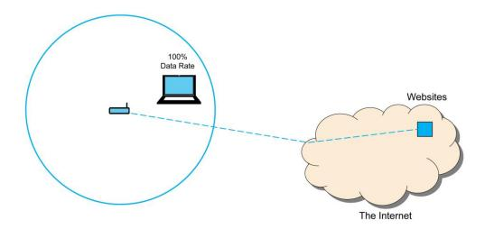
The following is a highly simplified description of how the user watches video from a website on their computer over Wi-Fi: User 1 clicks on a link on a website 1 to request a video stream, the website sends the data for that video to AP 1, then AP 1 modulates the data (i.e. creates a waveform that contains the data) as a radio signal and transmits that radio signal through the air. User 1's computer receives the radio signal, demodulates the data, and plays back the video.
