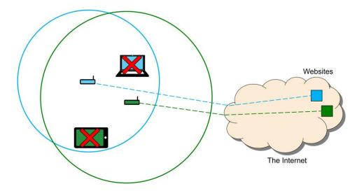
Interference caused by the 2 simultaneous Wi-Fi transmissions is shown by a red "X". Wi-Fi has several techniques to deal with interference, but the net effect is that they all share the channel, and as a result, reduce each user's data rate. For the sake of explanation, we'll show how very simplified spectrum sharing works, with each user taking turns. First User 1 uses the spectrum while User 2 stands by idle:
