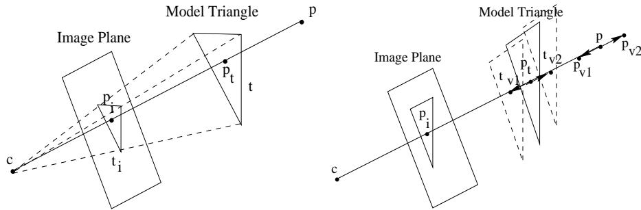
Figure 2: One dimensional visibility test. (a)Model's triangles and features are tested for 2D overlap in the image plane. (b)Representation of 1D variance of  $p, p_t$  along the projection optical ray.
