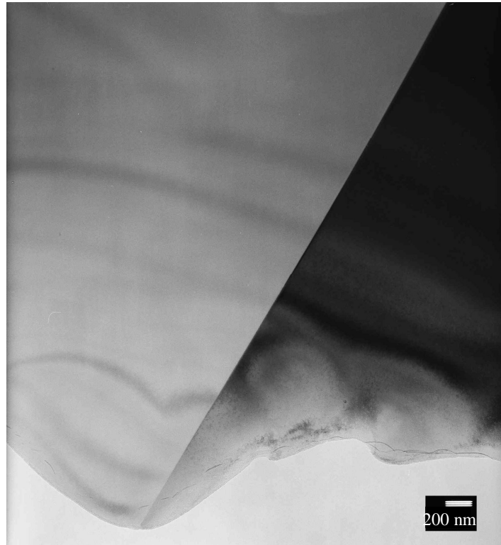
Figure 5.25. TEM micrograph of a grain boundary in an MLA-type sample.
