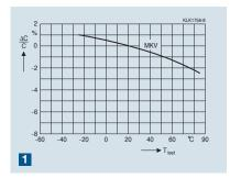
Relative capacitance change  $\Delta C/C$  versus test tmperature  $T_{test}$
