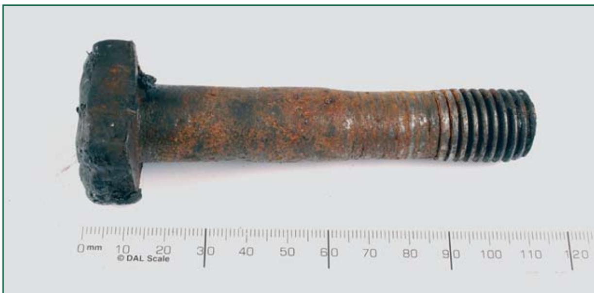
Figure 14: Lock stretcher bar bolt showing progressive thread damage
