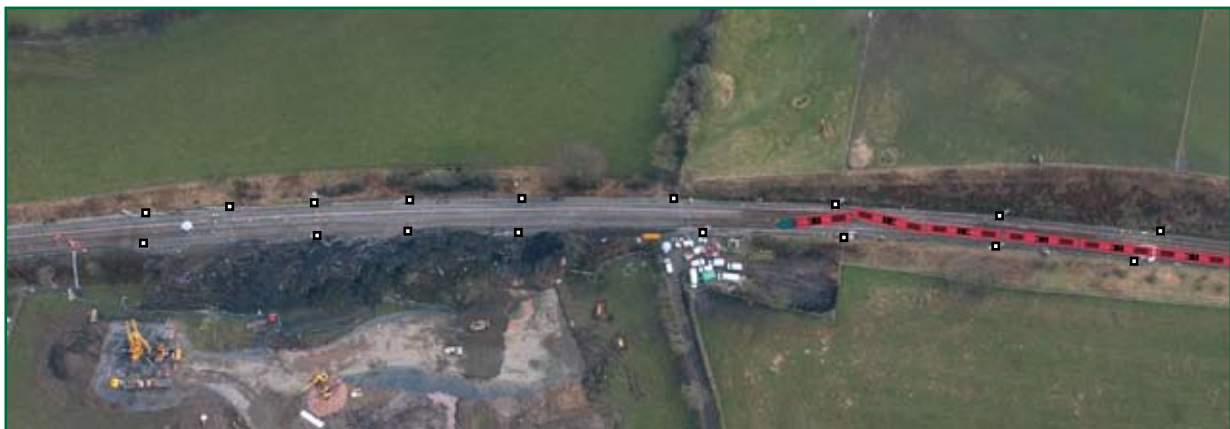
Figure 33: Diagram of the misalignment which developed between vehicles one, two and three after passing 2B points
