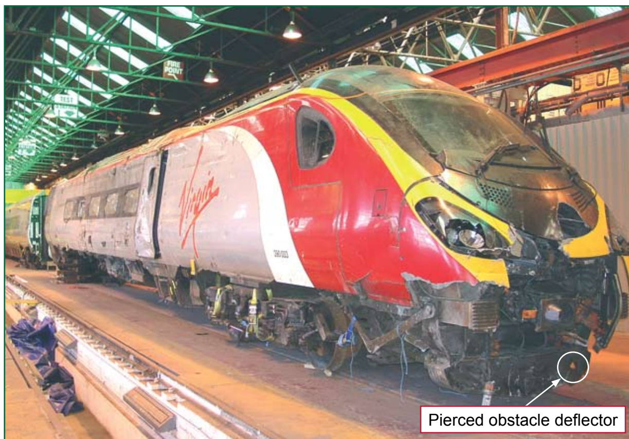
Figure 37: Damage to the right-hand bodyside of vehicle one and obstacle deflector
