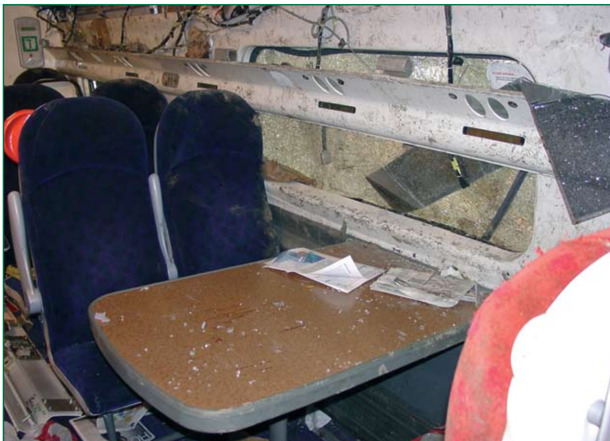
Figure 39: Detached reading light panels in the leading right-hand side of vehicle one
