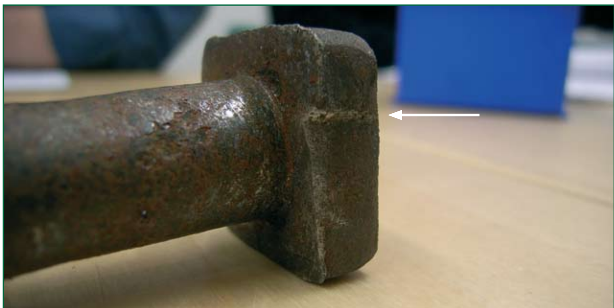
Figure 13: Indentation in lock stretcher bar bolt head
