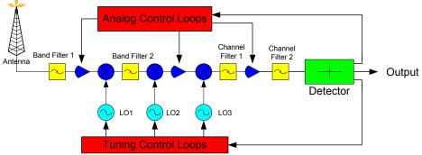
Figure 2: Traditional Super-heterodyne with analog detection
