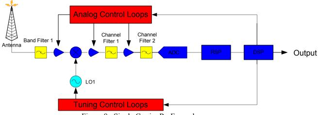
Figure 8: Single Carrier Rx Example
