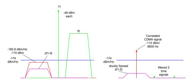
Figure 18: UMTS Intermodulation Performance Requirements
