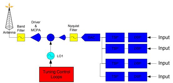
Figure 9: Multi-channel transmit with single up-convert super-heterodyne
