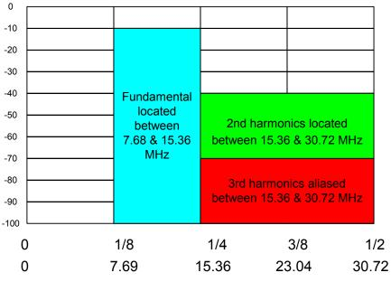
Figure 11: Aliased wideband signal and harmonics
