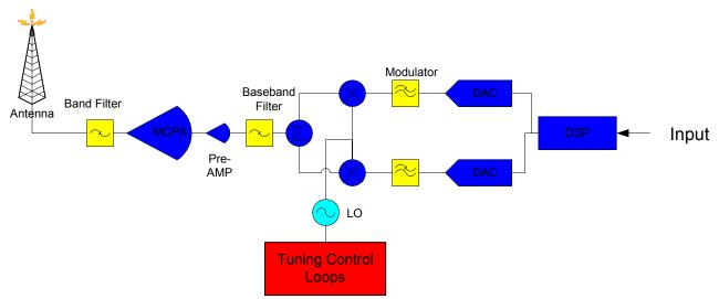
Figure 10: Single carrier direct conversion transmit
