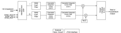
Figure 14: Fixed Function Transmit Signal Processor (TSP)
