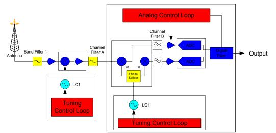
Figure 3: Super-heterodyne with baseband IQ sampling.
