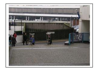
Eastern Square & Odeon walkway – currently a mix of untreated concrete and painted surfaces. It is proposed to be painted light grey with the exception of wall 5 which is part of a new structure (the Odeon walkway) and proposed to be plate glass and metal framing (see description of wall 5 below in section 3).
