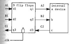
Figure 3: System Consisting of Flip Flops and an Internal Part
