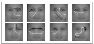
Figure 7. The first 8 features of the cascade. Each of them also acted as a non-face rejector. For illustration, the background is the mean of all the face patches in the training set.
