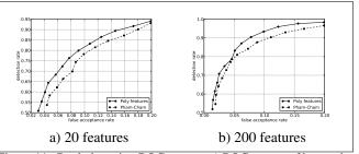
Figure 11. Rock detection ROC curves: a) ROC curves of boosted classifiers with 20 features, and b) ROC curves of boosted classifiers with 200 features.
