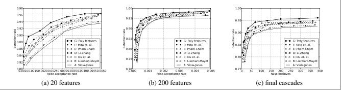
Figure 6. Face detection ROC curves: a) ROC curves of boosted classifiers with 20 features, b) ROC curves of boosted classifiers with 200 features, and c) ROC curves of the final cascades.
