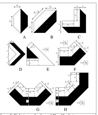
Figure 5. Eight types of polygonal Haar-like features were used in addition to Viola-Jones' four types of Haar-like features [24]. They were parameterized by  $(x, y, \theta_1, \theta_2, [\theta_3])$ . Scaling and translation were naturally incorporated in these parameters. Features were generated from these types, rotated by multiples of 90°, and mirrored. After all duplicate features were removed, a total of 210,366 features formed a polygonal feature pool.
