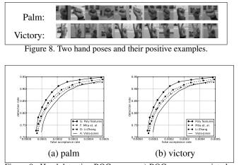
Figure 9. Hand detection ROC curves: a) ROC curves associated with the palm pose, b) ROC curves associated with the victory pose.
