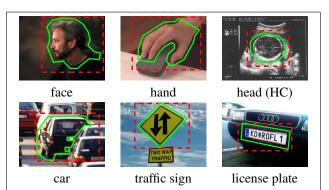
Figure 1. Some common targets for object detection. If the region of interest is known, it may be better to use a polygon than a rectangle to approximate the domain of integration, as more unwanted area can be avoided. With this work, fast integration over a polygonal region is possible, in time independent of the image resolution.
