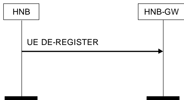
Figure 7 UE De-Register Procedure: HNB Originated Successful Operation
