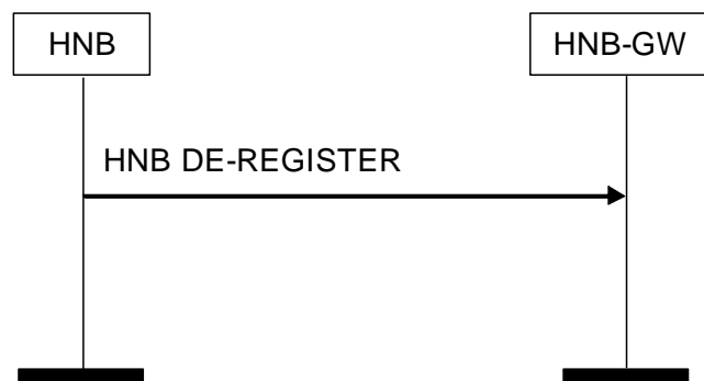
Figure 3: HNB De-register Procedure: Successful Operation
