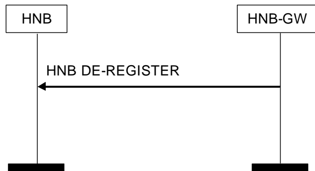
Figure 4: HNB De-register Procedure: Successful Operation
