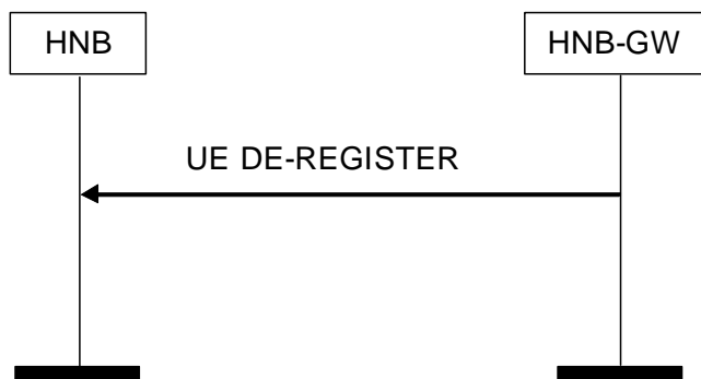
Figure 8 UE De-Register Procedure: HNB-GW Originated Successful Operation
