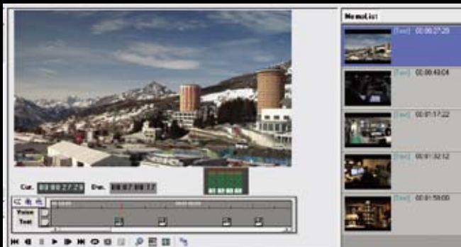
This shows the text memo editing window of the provided Windows PC software, P2 Viewer. A list of memos is shown on the right side. The clip time line below the view window shows the memo marks. Text can be written to an empty memo space created by the camera-recorder. Memos can also be added, deleted or moved.
