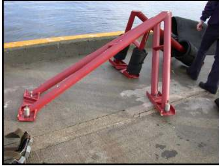
Figure 9 - Vector/EM1002A transducer protection grids (cow catcher)
