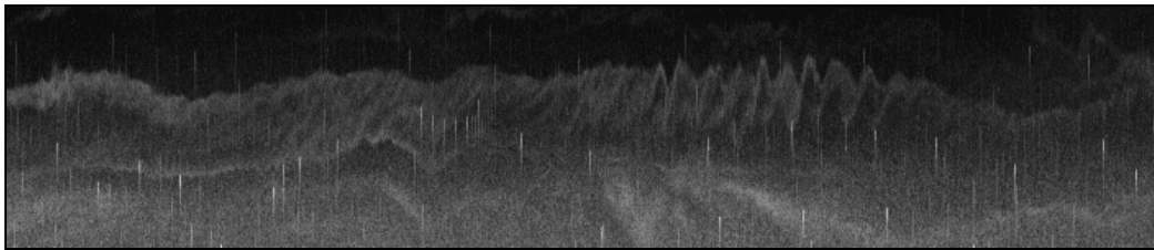
Figure 14 – EM710 water column imaging - internal waves off Race Rocks, Victoria
