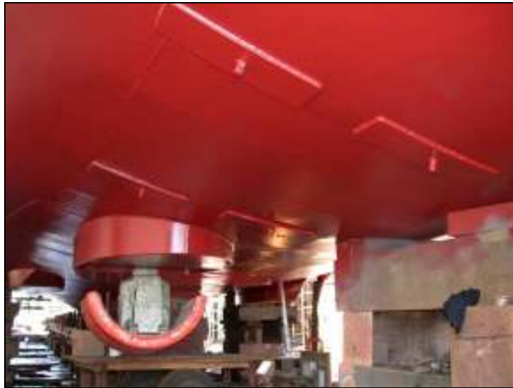
Figure 10 - Vector EM1002A installation on ram (Note studs for cow catcher)
