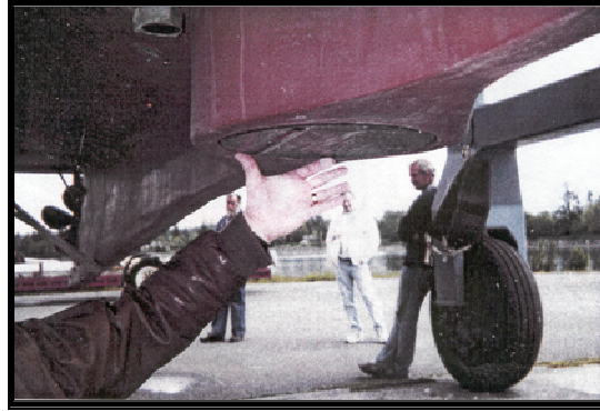
Figure 2 - Puffin in-keel fairing of EM3000
