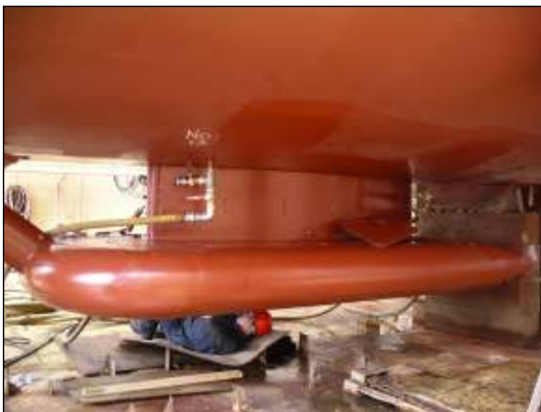
Figure 12 - BMT gondola design 2, as modified by Allied shipyard with additional CCG input
