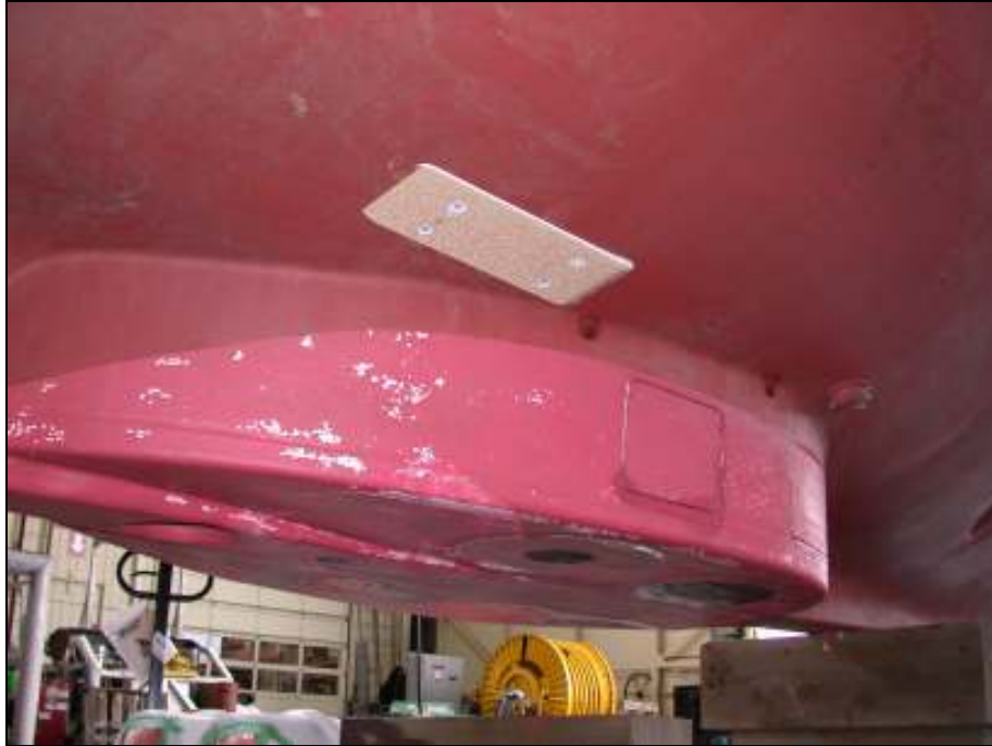
Figure 5 - Otter Bay along-keel transducer pod (EM3002 is on port forward)
