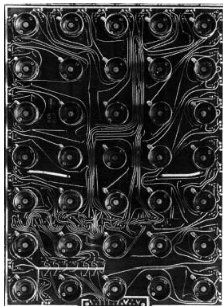
Wiring in a light chamber
