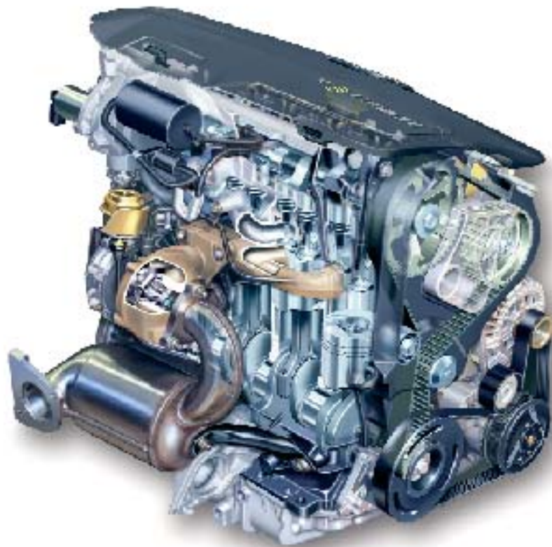
The 1.9-liter dCi is Renault's most versatile engine, with different versions generating from 80 to 120hp.
