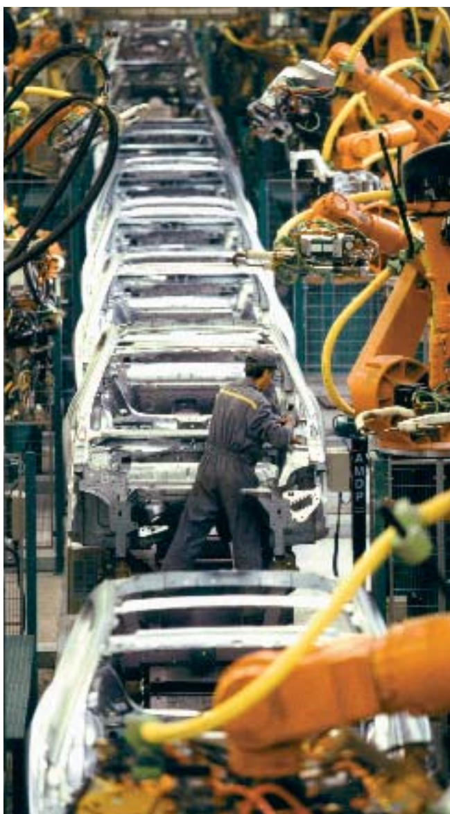
Mégane II Hatch shaping up on the body assembly line at Douai, France.
