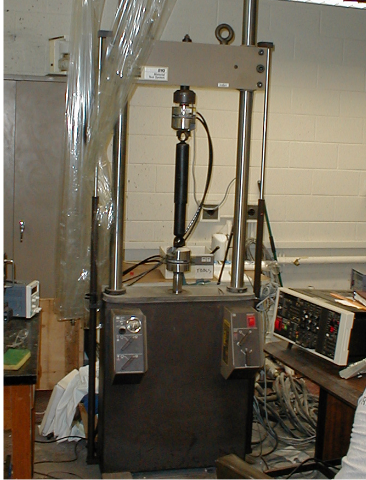
Figure 11. MTS machine used for automotive damper testing.
