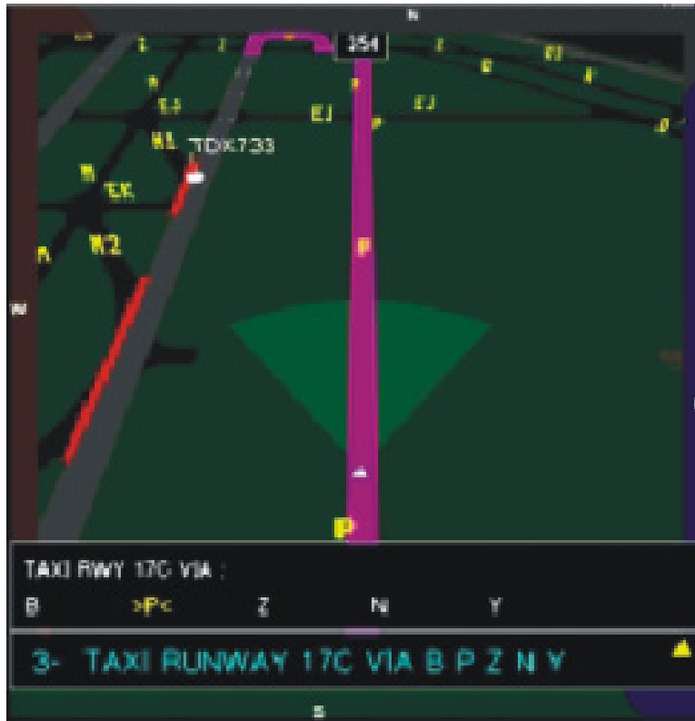
Figure E-6. Cockpit departure moving map display
