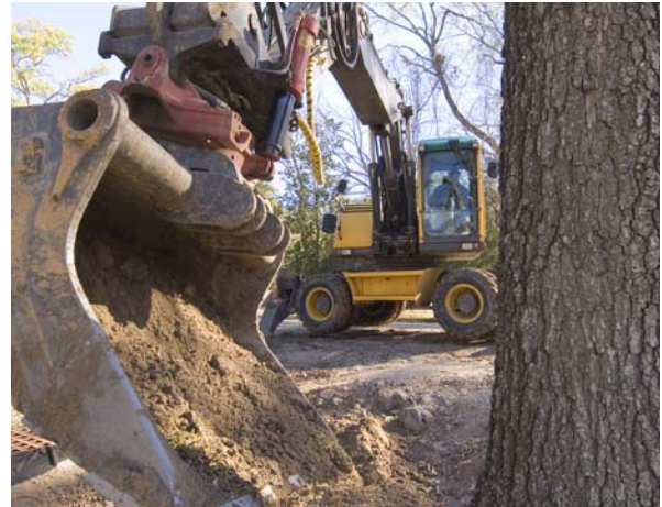
The Rototilt rotates 360° and tilts 40° and is very easy and smooth to operate with the unique Volvo factory installed Rototilt preparation kit.
