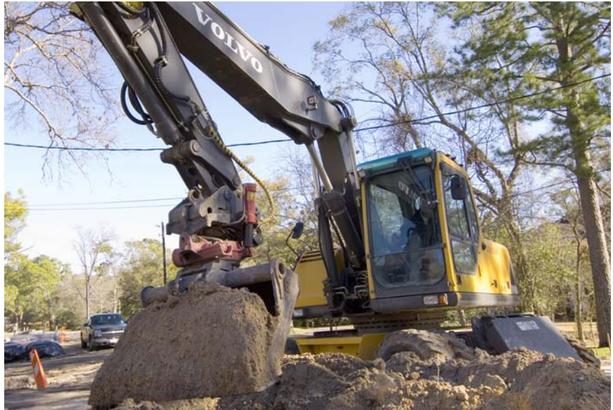
Barker says there is nothing like the versatility of a Volvo EW180B with a Rototilt attachment.
