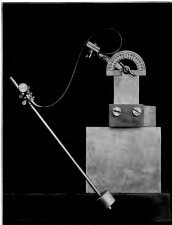
Figure 16: Born's experimental apparatus for measuring the elastica.
